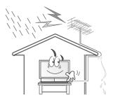
Any necessary action such as making the antenna cable loop at the entrance of the building should be taken to prevent rainwater on the outdoor antenna cable from possibly running into the indoor.
